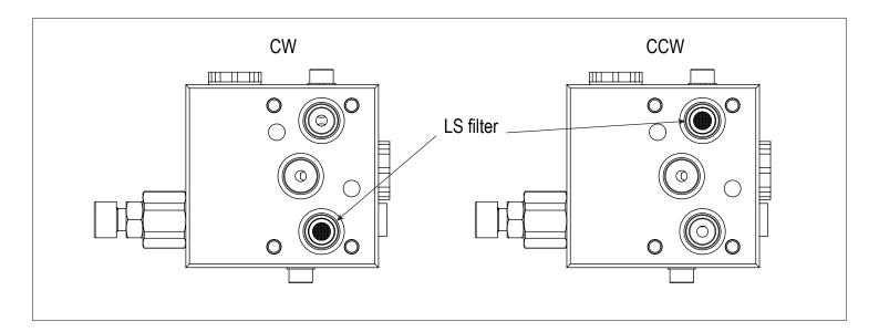
As all types of filtration, the LS filter requires regular maintenance to avoid clogging.
